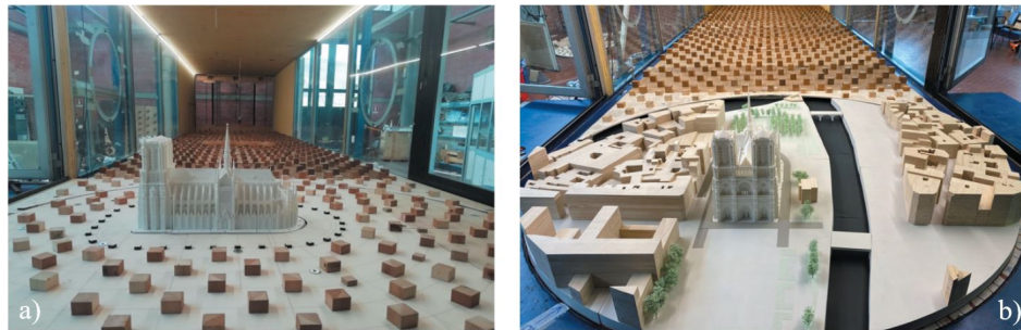
Figure 2. Model of the Cathedral in the wind tunnel without ( left ) and with ( right ) surrounding.
